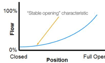
**Figure 2** - Flow characteristics of the venturi valve
